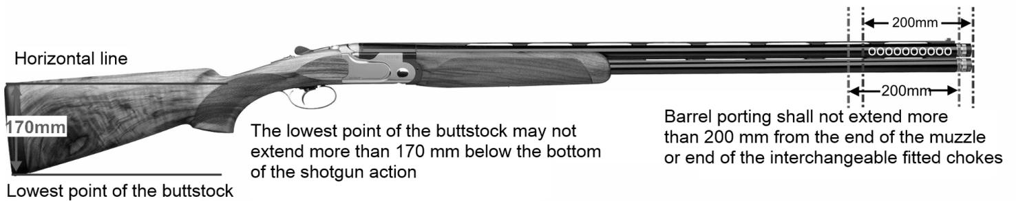
The lowest point of the buttstock or toe of the butt plate may not be more than 170 mm below a horizontal line extending from the bottom of the shotgun action (see illustration).
